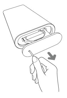
**3** Place the supplied CR2025 battery into the tray. Ensure the "+" symbol is facing upwards.
